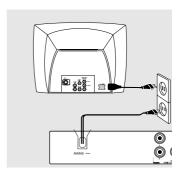
After everything is connected properly, plug in the AC power cord to the power outlet.
